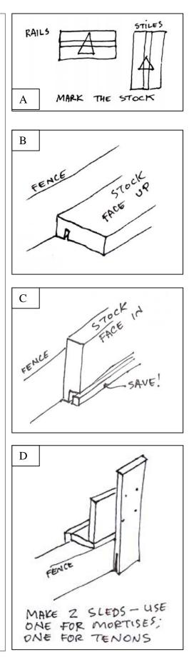
this 1/8" kerf/mortise, set the fence to 3/8" (a lateral move of 1/8". Use the same jig, and make a second pass with the stiles. You will now have a bridle joint mortise 1/4" thick.
