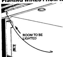
Gut an access hole in wall about 6 in. below selling (save cutout for following repair) Bore hole in top plate. Insert fish tape.
