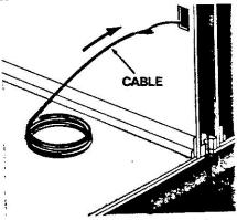
Attach cable to hooked end of the fish tape. Wrap connection with electrical tape and pull it through wall opening into basement.
