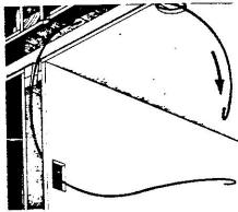
Withdraw the ceiling-hole tape until the booked end of the electrical box tape is in band. Attach cable to the other end of tape and pull it through to the ceiling hole.
