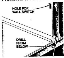
Working from below, bore a hole through the bottom plate of the wall into the wall cavity where wall switch is to be located.
