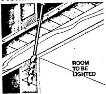
Remove the baseboard in the room above to bore a hole through the wall's top plate. Bore diagonally, as shown, using a brace and a %-in.-dia. x 18-in.-long bit.
