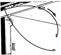
Feed a second tape through the colling hole and maneuver both until you are able to hook the two tape ends together as shown.
